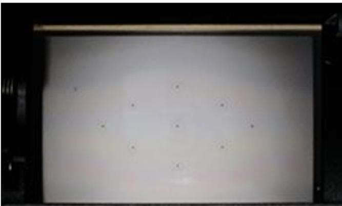
The mirror is unique to DSLR cameras. It reflects light from the lens into the viewfinder, which lets the photographer see the shot through the viewfinder in real time. The mirror flips up immediately right before shutter release (the shot is taken).
