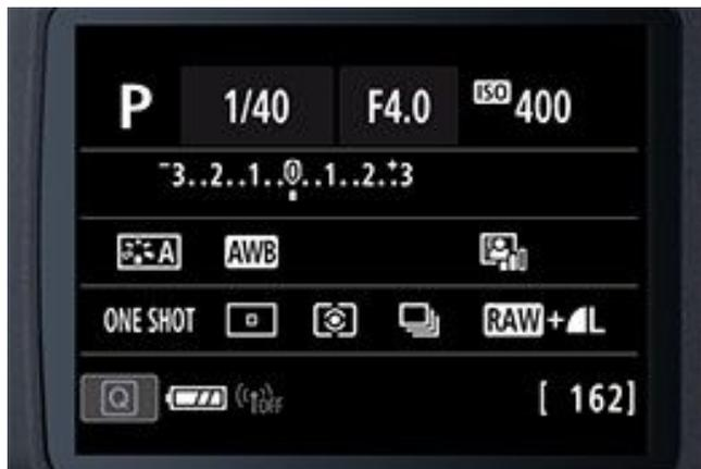
In addition to the shooting settings as shown in the illustration here, the captured image as well as text information such as the menu can also be displayed on the LCD monitor. Also, you can magnify the display image to check the details. Some camera models have a Vari-angle LCD monitor, which allows you to alter the angle of the monitor during Live View shooting, making it easier to capture low-angle or high-angle shots.
