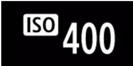
A higher ISO speed makes it easier to capture shots of a dimly-lit scene. Generally, ISO 100 is used as the standard setting. In the ISO Auto setting, the optimal value is automatically selected according to the scene. You can also choose to set the ISO speed manually.
