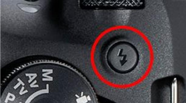
Use this button to pop up the built-in flash. In the Basic Zone, the built-in flash may pop up automatically in some cases according to the function in use.
