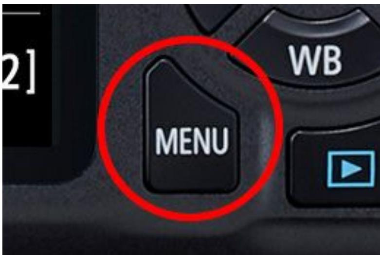
Use this button to display the menu for adjusting the different camera functions. After selecting a menu item, you can adjust the camera settings in greater detail.
