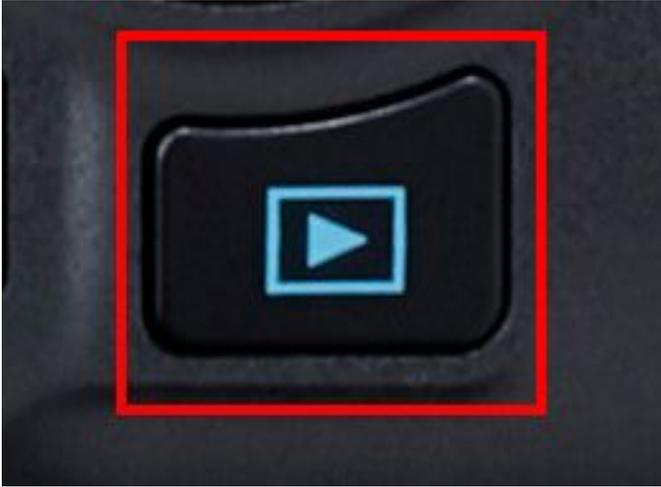
This is the button for playing back images you have captured. Pressing the button once displays the last image you captured or showed on the LCD monitor.
